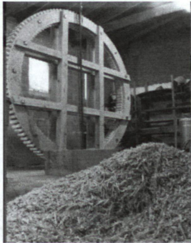
Spur Gear- 9ft. 2in. Diameter, 122 cogs- White Oak, Rock Maple Bowmansville Mill- Lancaster Co., PA
