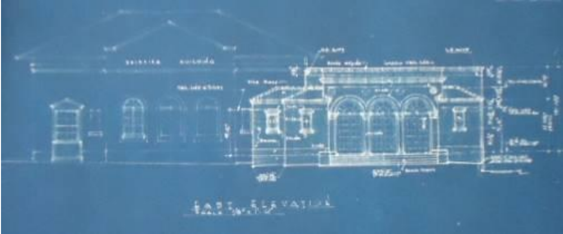
Figure 11: East elevation of Waples Hall (right) as it ties into Anna Shelton Hall (left). The building that was constructed did not have arched entrances to the portico as depicted in this drawing. W. G. Clarkson & Co., architect, 1949. Courtesy TWC.
